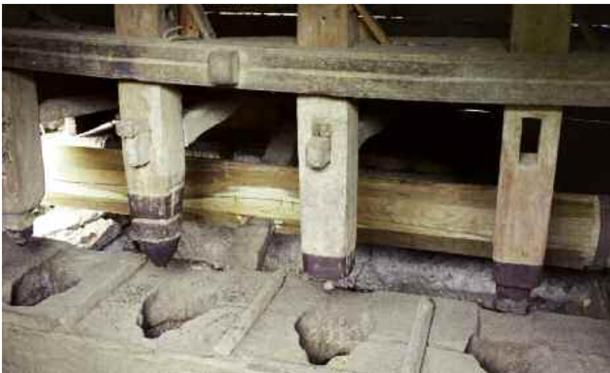
Stope na vodni pogon / Water-driven buckwheat dehusking device
